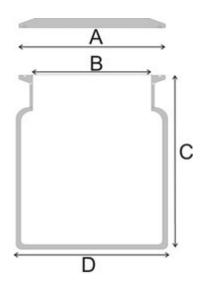
Method of Construction: Crevice free interior, welds ground & polished
